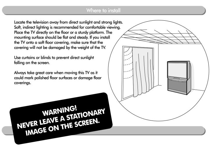
If stationary images generated by TELETEXT, CHANNEL IDENTIFICATION LOGOS, COMPUTER DISPLAYS, VIDEO GAMES, ON SCREEN MENUS, etc. are left on the TV screen for any length of time, they will become permanently ingrained.
